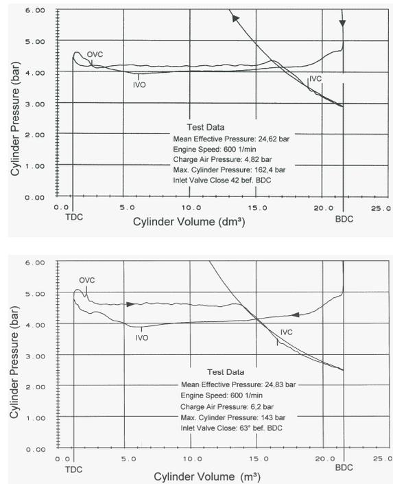
Figure 6: Low pressure p-V-Diagram Miller 42 and 63
