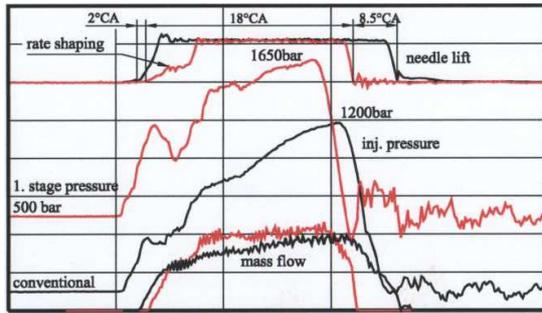
Figure 2: Influence of First stage pressure on line pressure, needle lift and mass flow
