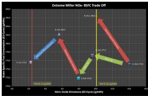
Figure 10: Concept for optimized IMO Tier II and Tier III engine layout
