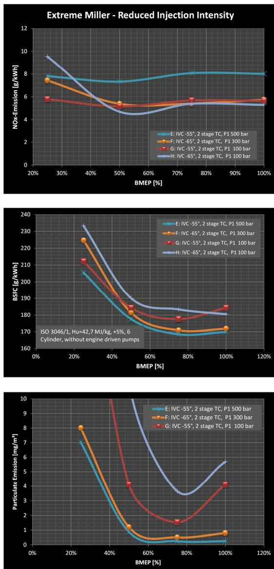
Figure 7: Influence of injection intensity at extreme miller configurations
