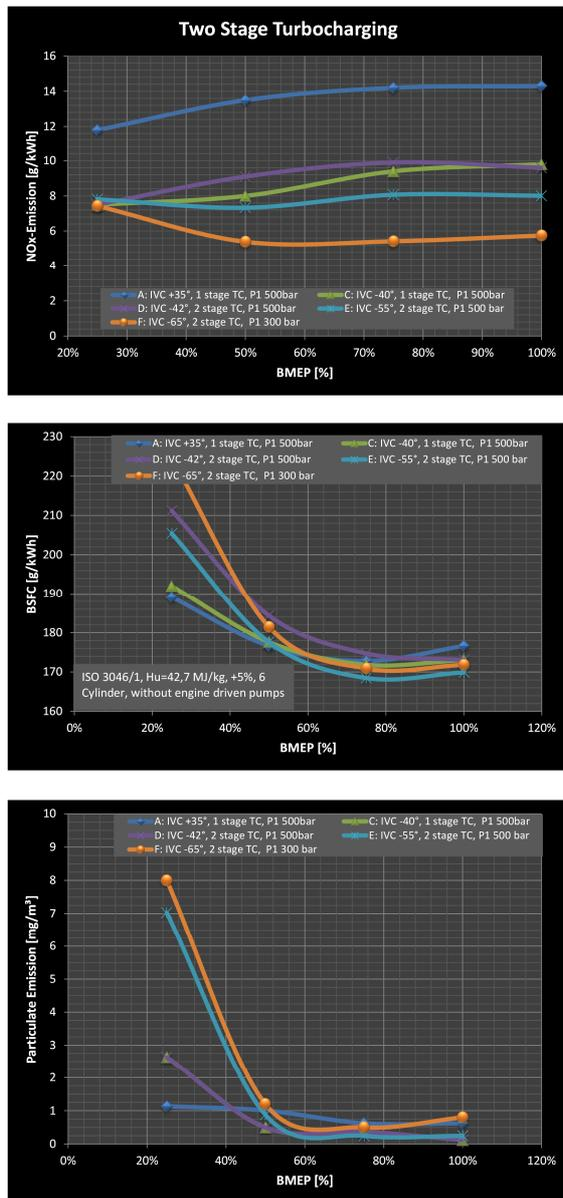
Figure 5: Comparison of extreme Miller test results
