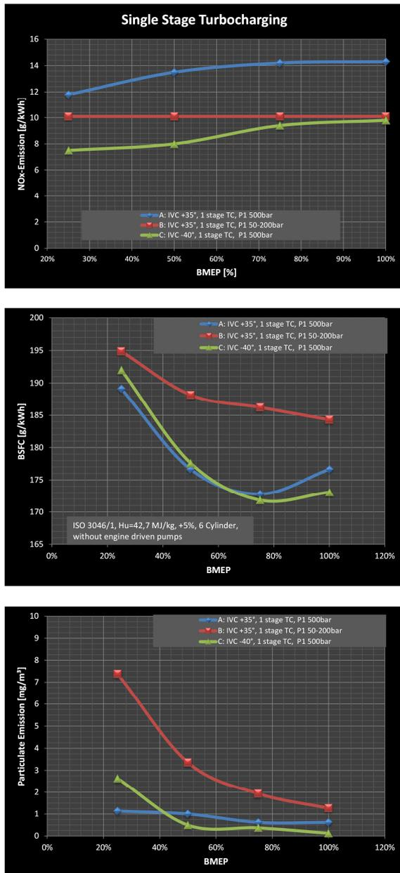
Figure 4: CLEAN I test results
