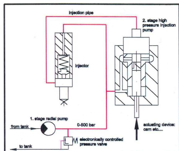
**Figure 1: Two stage injection system**
