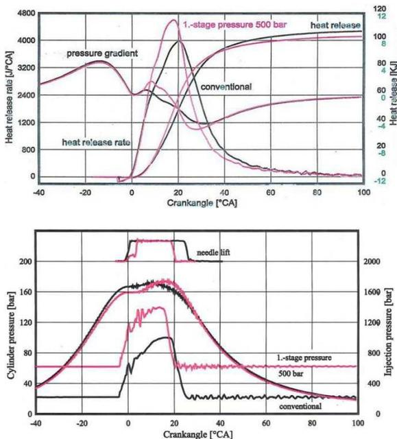
Figure 3: Influence of first stage pressure on injection and combustion characteristic
